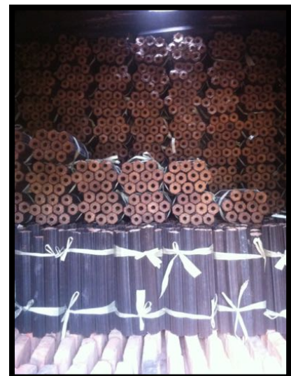
Sawdust Extruded Wood Briquettes for Charcoal Processing
