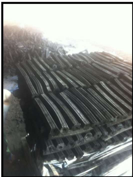
Sawdust Extruded Wood Charcoal – cooling process after cooking in ovens.
